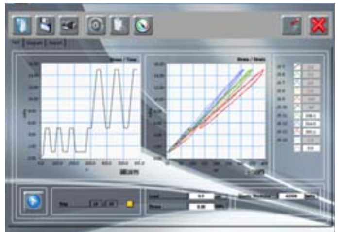
E-MODULE software: Elastic Modulus test performed according to EN 12390-13 (Procedure A)
