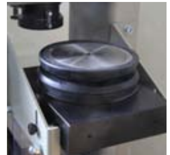
Detail of the upper block platen and spherical seat sliden off on the solid rail system, to fit the platen assembly for testing cylinders
