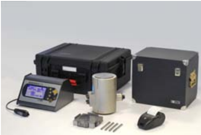
82-P0804/E with 82-E0105/1 Strain gauged column and 82-P0172/M 24 column printer. The strain gauged column is supplied complete with auxiliary platen and spacers for an easy and precise placing of the column either centrally or 6 mm displaced from the centre. It can also be used as a 3000 kN load cell for force verification.
