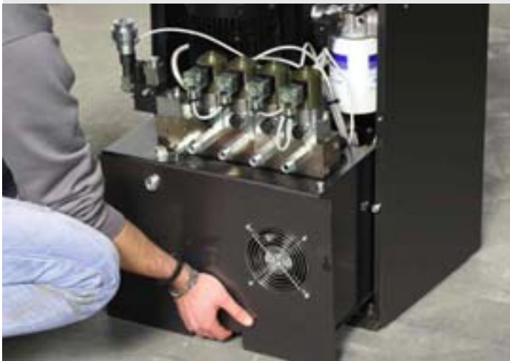
Rear view of the MCC Power and Control Consoles. The four hydraulic ports for connection of test frames are visible (the MCC has two ports, extendable to four)
