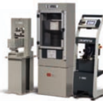
DIGIMAX 3 SMART-Line, stand-alone control console 50-C10B02 with 50-C56Z00 frame and distribution block 50-C10B/2F for the control of 50-C0910/FR flexure frame
