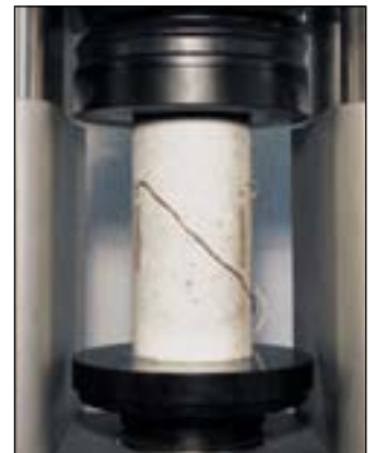
Concrete specimen fitted with Strain Gauges
