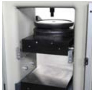
Detail of the sliding off operation of the upper block platen and spherical seat, to be replaced by the platen assembly for testing cylinders.
