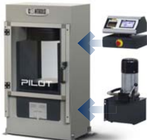
PILOT Automatic Power and Control system, connected directly to a compression frame. The display unit is upgraded with the serial graphic printer 50-C10B/PR
