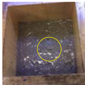
Micro-chip (LF technology) cast into the fresh concrete
