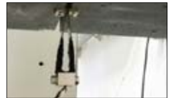
First Crack CMOD test
