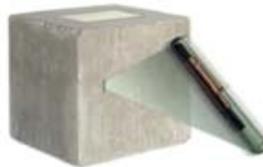
Micro-chip (LF technology) is permanently locked inside the hardened concrete specimen
