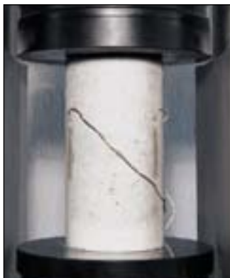
Determination of Elastic Modulus using surface-mounted Strain gauges
