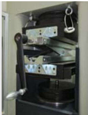
Detail of the compression frame fitted with lifting device 50-C9060/B.
