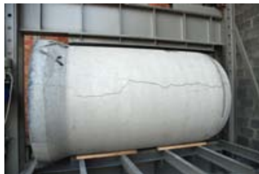
Large concrete pipe tested with the 50-C9602 machine
