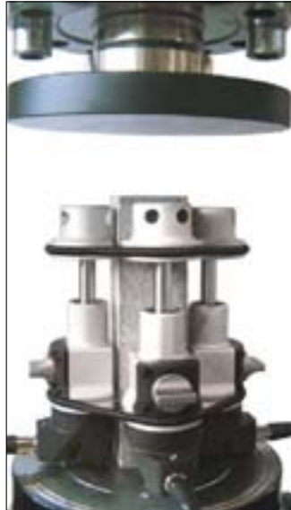
Three compressometer-extensometers (55-C0222/F) fitted to a cement prism 40 x 40 x 160 mm
