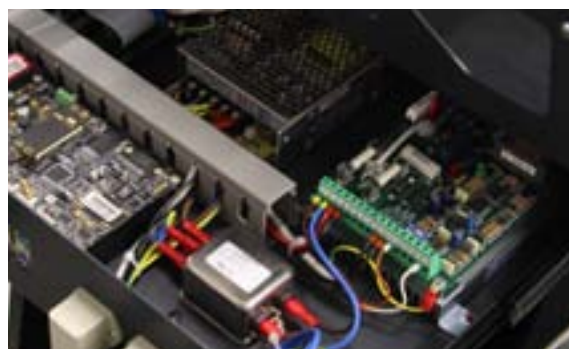
Detail of electronics positioned in the sliding drawer of Automax E-Modulus Console
