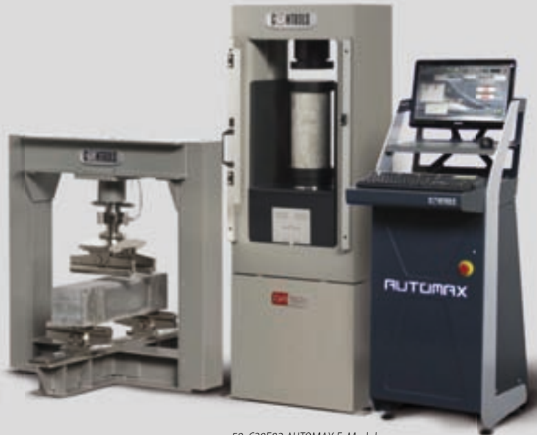
50-C20E82 AUTOMAX E-Modulus controlling a 2000 kN ASTM compression frame 50-C42Z00 and a 100 kN flexure frame 50-C1201/BFR with accessory.
