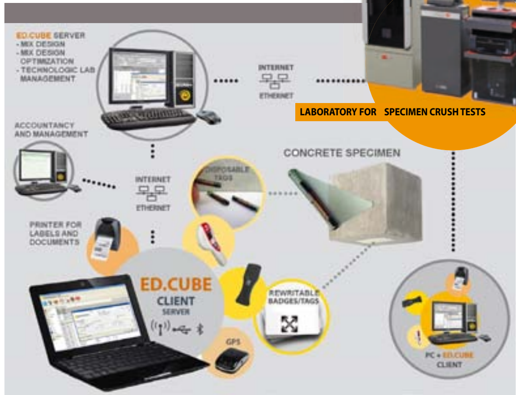
Layout of a complete system for concrete traceability
