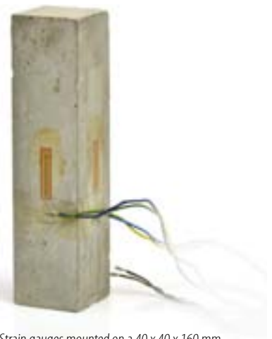
Strain gauges mounted on a 40 x 40 x 160 mm mortar prism
