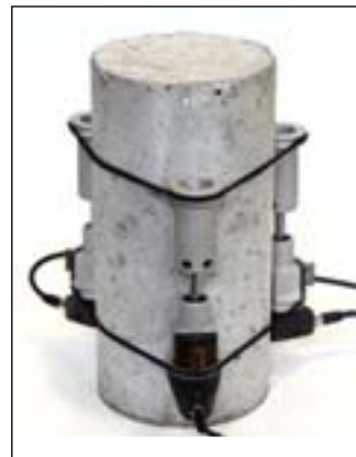
Concrete cylinder fitted with three Compressometer-extensometers 50-C0222/F
