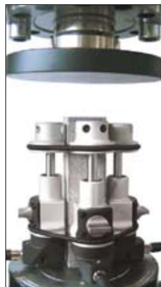
Concrete cylinder fitted with three Compressometer-extensometers 50-C0222/F
