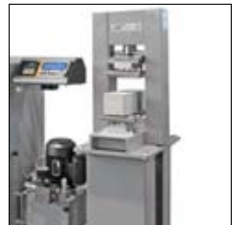
Upgrading of the power pump by a two way valve to connect a second frame
