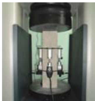
Three compressometer-extensometers 55-C0222/F fitted to a concrete beam
