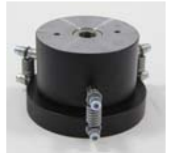
Detail of upper platen and spherical seat strictly conforming to ASTM C39 and AASHTO T22
