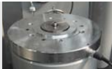
50-C86Z10 Detail of load cell housed in the ram
