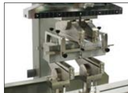
Detail of the auxiliary frame and specimen
