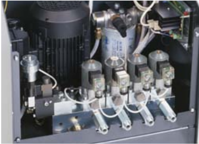
MCC console upgraded with 50-C7022/UP2 distribution block for connection to up to 4 frames
