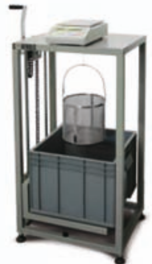
11-D0612/B with 11-D0612/1 Density basket and 11-D0630/30 electronic balance
