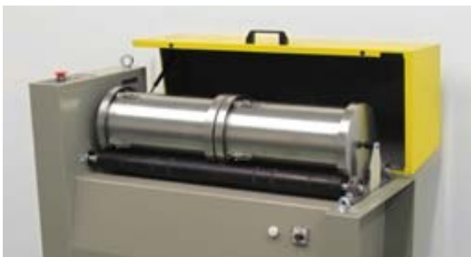
48-D5242 with two 48-D0524/8 cylinders, 200 mm diameter, 400 mm long
