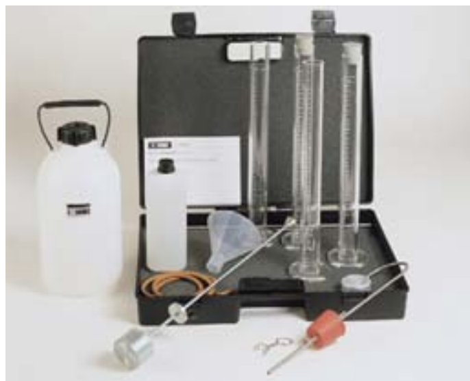
47-T0050/B with 47-T0050/7. The 47-T0050/C version is identical except for the graduation of the cylinders and some small differences in the weighted foot.
