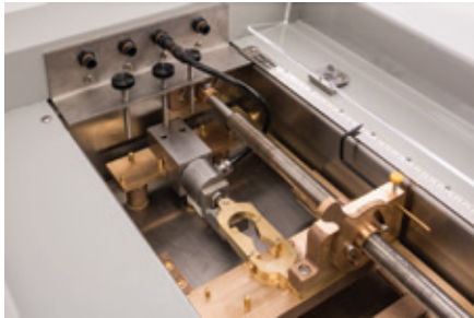
Interior of HA-1060 showing force determination transducer set up.
