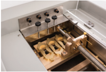
Interior of HA-1060 showing test molds, screw drive and disengage lever.
