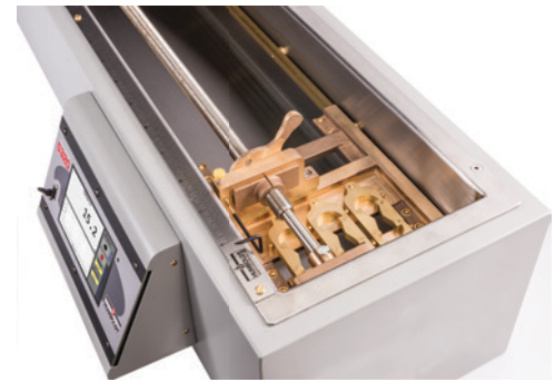
Interior of HA-1068 showing test molds, screw drive and disengage lever.
