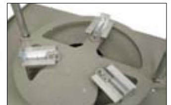
Detail of the adjustable base for 200 to 450 mm diameter sieves
