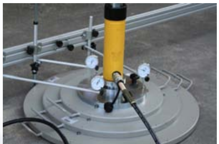
Set of load plates, dial gauges, dial gauge supports and datum bar (partial view).
