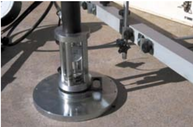
35-T1170, 35-T1170/D, Detail of dial gauge housing conforming to CNR N° 146 method A standard
