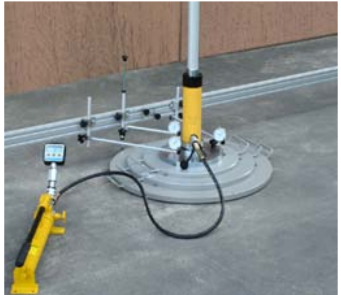
35-T1173/D detail of plate set, hydraulic cylinder, dial gauges with supports, hand pump and high resolution digital gauge: 0-200kN range, 10N resolution.
