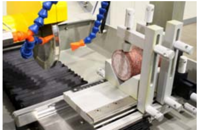
45-D0536/A, detail of spindle with clamping mechanism and double-faced cup wheel 45-D0536/A3 during surface grinding of cylindrical specimen ends
