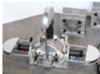
45-D0548/D: Detail of the shear box apparatus fitted with 5 displacement transducers
