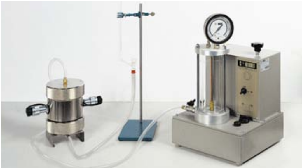
28-WF4312 with Hoek cell, Permeability end caps, burette, support base and metal/glass sleeve
