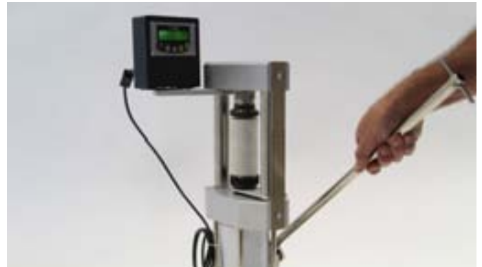
45-D0550/E fitted with set 45-D0550/D5 for compression test
