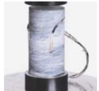
Detail of rock sample fitted with 3 strain gauges
