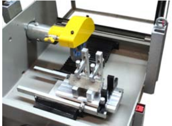
45-D0536/A, detail of spindle with clamping mechanism and cutting blade 45-D0536/2
