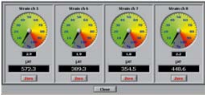
ADVANTEST, virtual gauges indicating the real-time readings of the sensors both in engineering units and as a percentage of the full scale. An excellent tool for transducer positioning.
