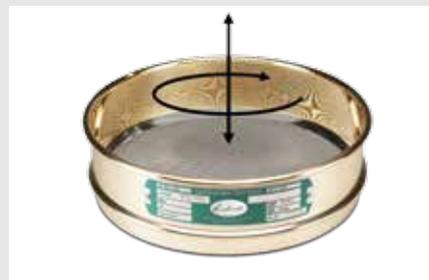
Vertical vibration is generated by the on/off frequency of the electromagnetic drive. However, vertical vibration is not enough to impart the correct movement for sieving. The shaker also needs to twist the sieve stack - this rotating action ensures the sample passes over the full surface of the sieve and the maximum number of apertures to give rapid accurate results
