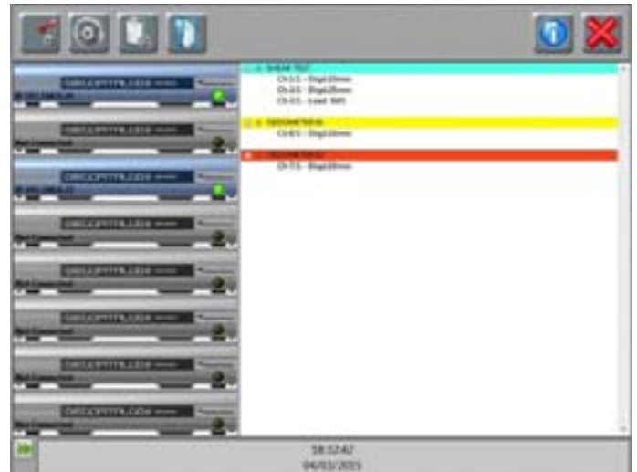
DATACOMM 2 - Channels configuration. The transducers can be grouped and combined by the user for matching different applications.
