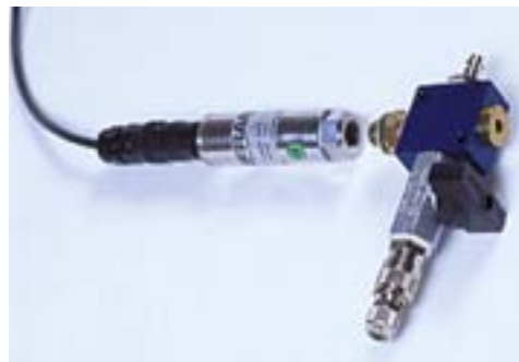
Pressure transducer 28-WF6300 connected to the de-airing block 28-WF6310 for banded triaxial cells.
