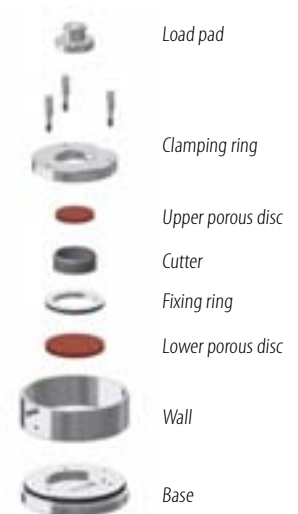
Exploded view of consolidation cell 26-WF0320
