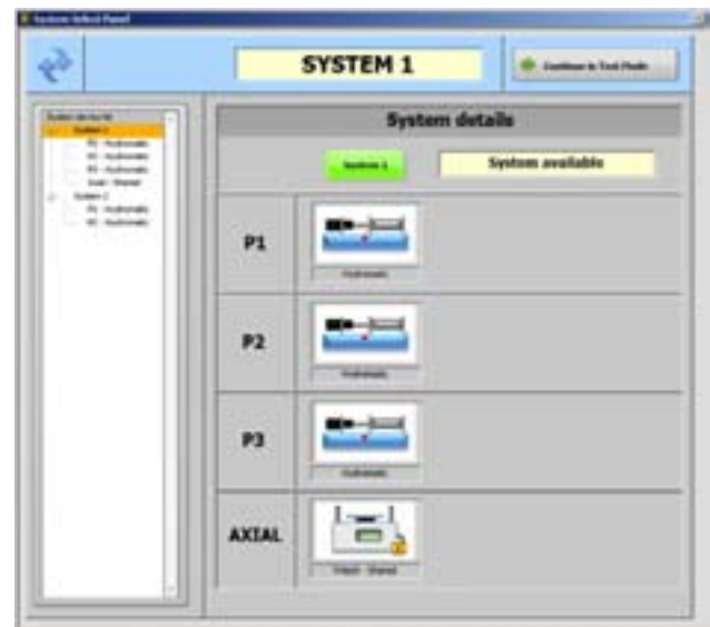
System Select panel showing two triaxial systems are available, with one shared Trittech compression frame, one system is suitable for permeability test
