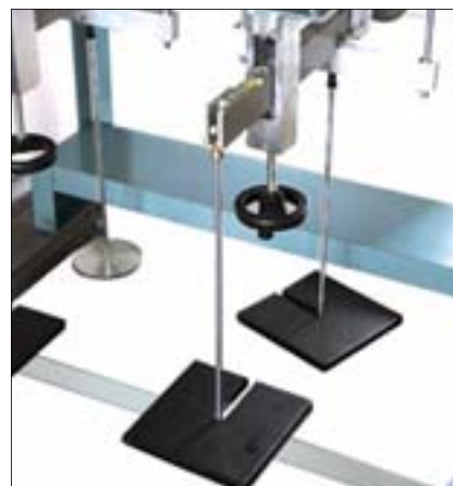
Detail of the 28-WF0493/3 beam loading device and slotted steel weights
