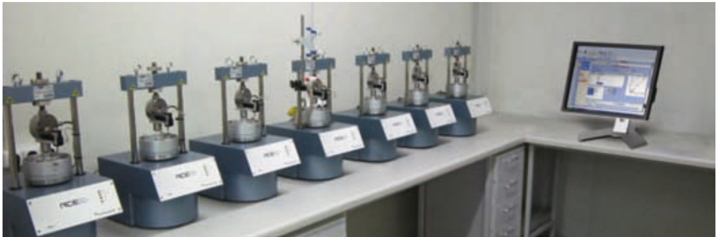
Modularity concept: up to 60 ACE units can be connected to the same PC via LAN and controlled by the same software 26-WF3120/SOF.
