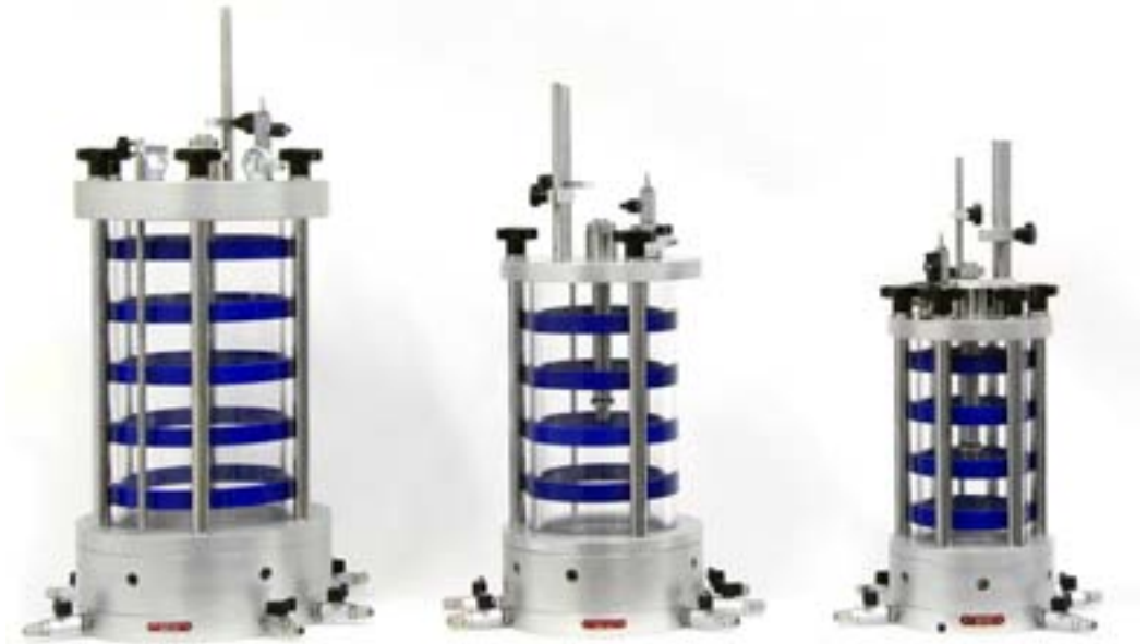
Banded triaxial cells fitted with upgrading kits for using local strain transducers and bender elements
