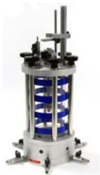
Banded triaxial cell 28-WF4070 fitted with upgrading kit 28-WF4070/ADV for using bender element and local strain transducers
