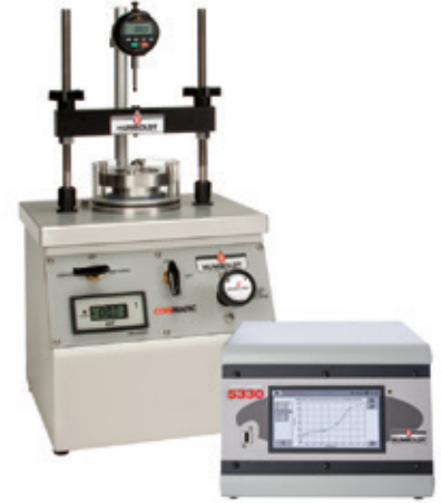
HM-2432A.3F shown with HM-5330.3F Data Logger for semi-automatic control and data acquisition with digital indicators.
