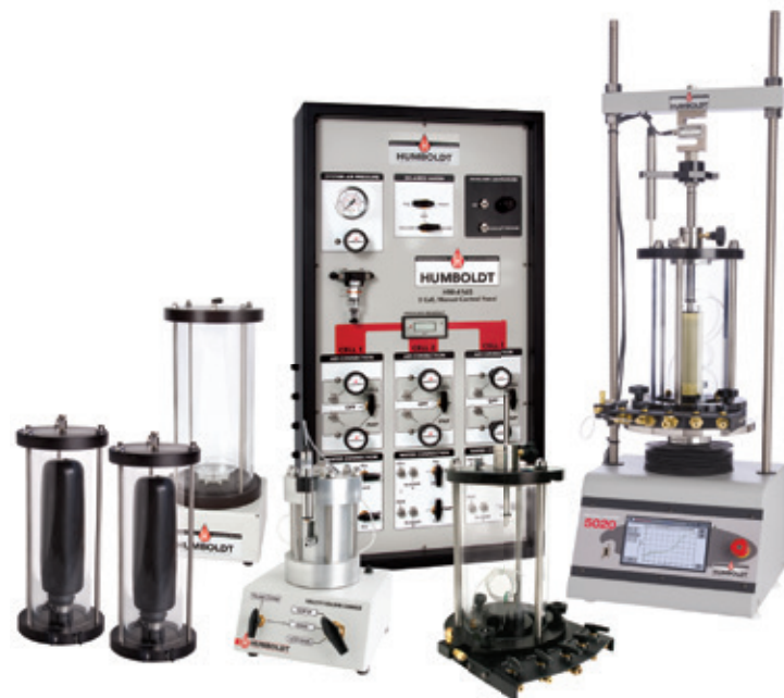
Manual Pressure Control Triaxial System Components
