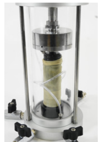
Detail of standard triaxial cell fitted with submersible load cell
