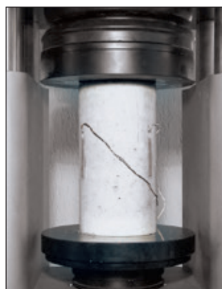
Determination of the Elastic Modulus using surface-mounted strain gauges
