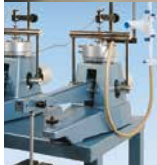
Three oedometers 26-WF0302, complete with cells, 30-WF6207 displacement electronic transducers connected to 30-WF6008 GEODATALOG, and 26-WF0312 consolidation bench.
