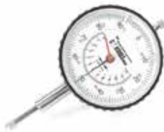
30-WF6401 Dial gauge for measuring vertical deformation, 12 mm x 0.002 mm resolution
