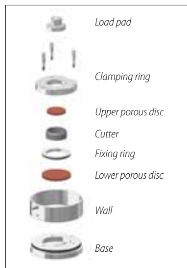
Exploded view of consolidation cell 26-WF0320
