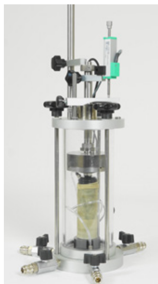
Standard triaxial cell, fitted with submersible load cell, displacement transducer
