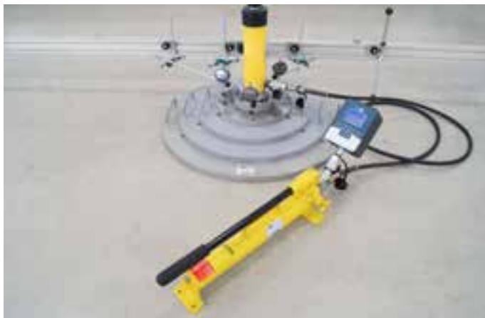
Detail of digital configuration with digital gauges positioned on the bearing plates
