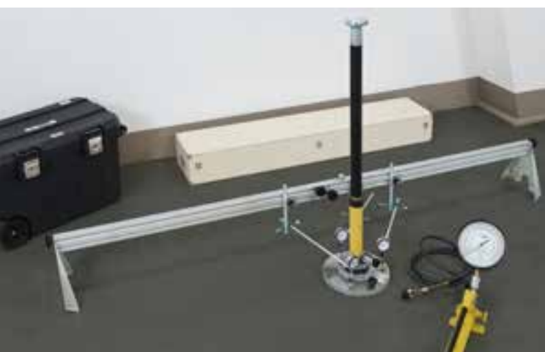
Model 35-T1101, analog version with manometer, 3 dial gauges and carrying cases
