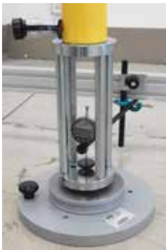
Measuring tunnel 35-T1100/MT suitable for single displacement device configuration
