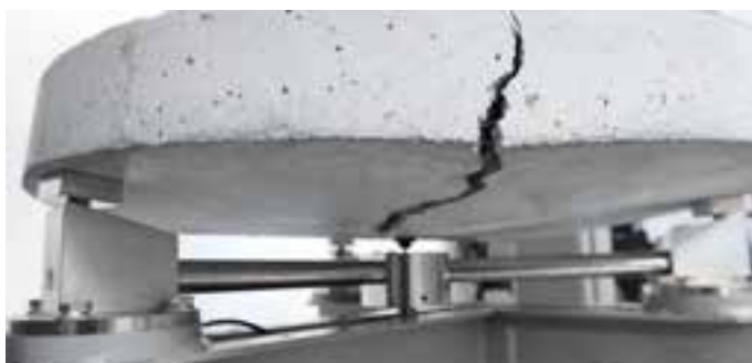
Slab testing to ASTM C1550 in 350kN SIMPLEX flexure frame 50-C1711/FR
