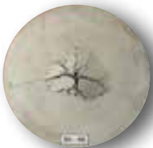
Round concrete slabs, 800 mm dia., subjected to concentrated load test to ASTM C1550
