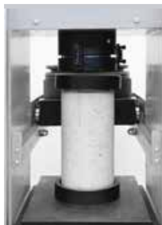
Detail of the machine fitted with the conversion set 50-A29/CYL to test cylinders
