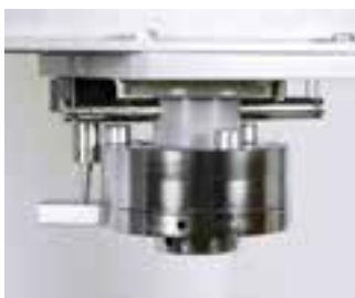
Detail of load cell and piston travel displacement transducer 50-C1500/9
