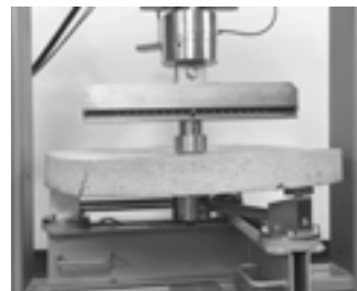
Slab testing to ASTM C1550 in 350kN SIMPLEX flexure frame 50-C1711/FR
