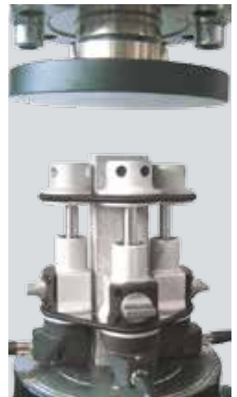
Three compressometer-extensometers 55-C0222/G fitted to a mortar prism 40 x 40 x 160 mm
