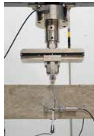
CMOD test to EN 14651 with CTOD measurement
