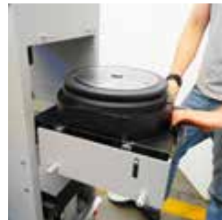
Detail of the upper block platen and spherical seat sliding off by solid rail system
