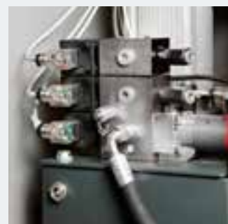
50-C10P/2F upgraded with third electrovalve 50-C10D/3F
