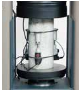
Three compressometer-extensometers 55-C0222/G fitted to a cylindrical specimen during compression stage.
