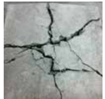
Square concrete slabs, 600x600 mm, subjected to concentrated load test to EN 14488-5
