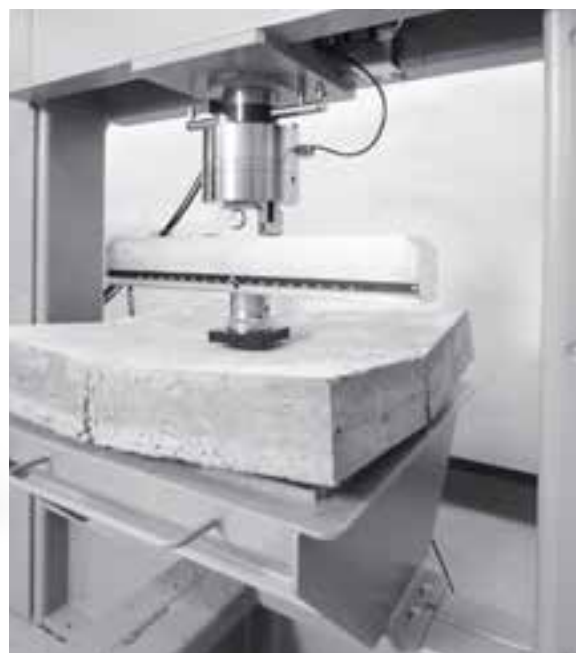
50-C1701/FR with C1500/6 and C1500/8 for square slab testing to EN 14488-5
