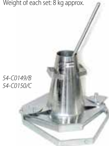
54-C0149/B, 54-C0150/C during use. The handle raises up over specimen and slump is measured using the tamping rod which is engraved with 1 cm graduations.
