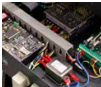
Detail of electronics positioned in the sliding drawer of Automax Multitest Console
