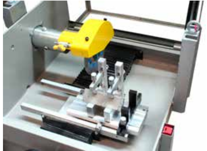
32-D0536/A, detail of spindle with clamping mechanism and cutting blade 32-D0536/2
