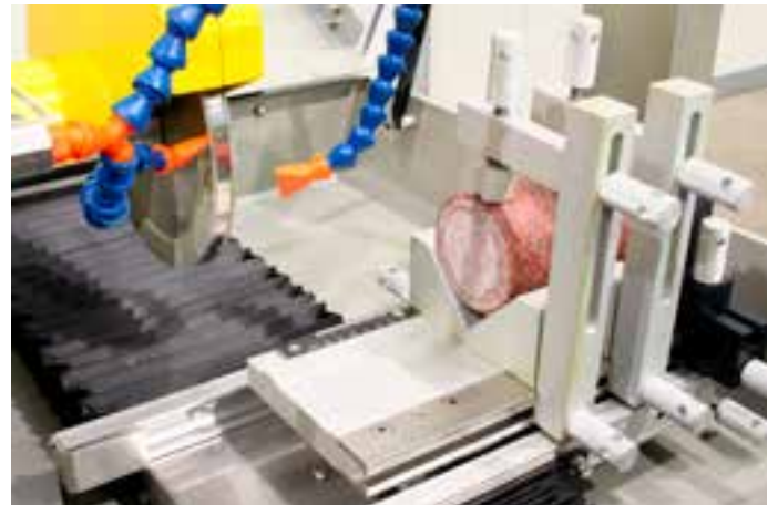
32-D0536/A, detail of spindle with clamping mechanism and double-faced cup wheel 32-D0536/A3 during surface grinding of cylindrical specimen ends
