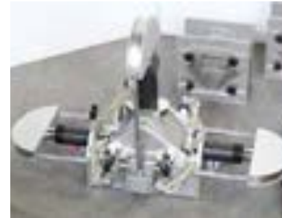
32-D0548/D: Detail of the shear box apparatus fitted with 5 displacement transducers
