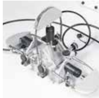
32-D0548/A: Detail of the shear box apparatus fitted with 5 digital gauges (4 vertical and 1 horizontal)
