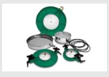
A wet sieving kit includes a top clamping plate with a Perspex cover and spray rose, watertight O-ring seals and a stainless steel receiver with drainage spout. O-ring seals may also be ordered separately.
