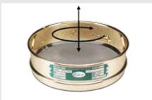
Vertical vibration is generated by the on/off frequency of the electromagnetic drive. However, vertical vibration is not enough to impart the correct movement for sieving. The shaker also needs to twist the sieve stack - this rotating action ensures the sample passes over the full surface of the sieve and the maximum number of apertures to give rapid accurate results
