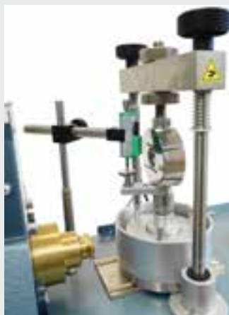
Detail of Shearmatic EmS fitted with Consolidation accessories and consolidation cell for automatic performance of the consolidation test
