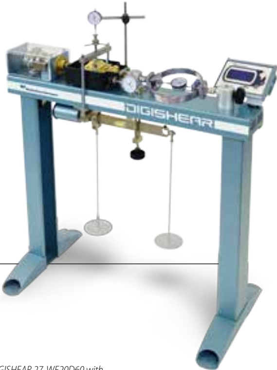
DIGISHEAR 27-WF20D60 with accessories, fit in the analogical mode.
