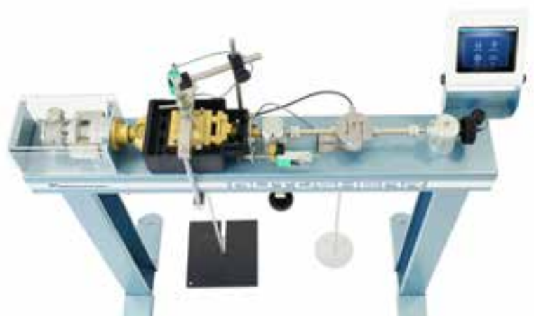
Detail of high stiffness load chain shear box - driving head - load cell
