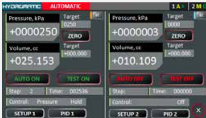
Auto Control: Automatic execution of pre-programmed steps of pressure and/or volume change
