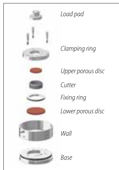
Exploded view of consolidation cell 26-WF0320
