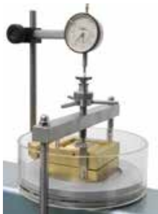
Detail of shear box case fitted in analog mode
