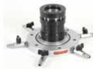
CRS - Constant Rate of Strain (26-WF0360/AD) fitted on lower base of banded triaxial cell.
