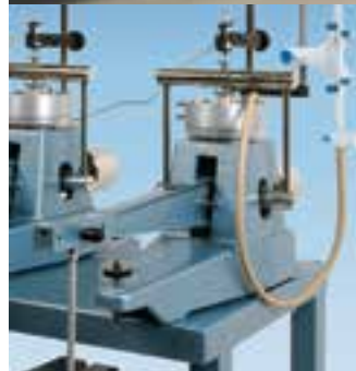
Three oedometers 26-WF0302, complete with cells, 30-WF6207 displacement electronic transducers connected to 30-WF6008 GEODATALOG, and 26-WF0312 consolidation bench and PC..
