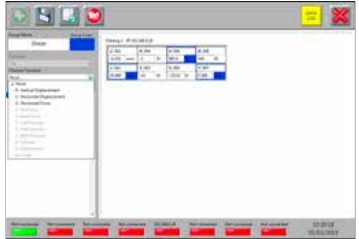
Channels (load cell, vertical displacement transducer and horizontal displacement transducer) and template assignment for performing direct shear test with real-time data processing using our Geo-Analysis templates
