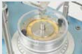
Detail of 40 cm 2 stainless steel ring shear box fitted with easily removable sintered porous stones with specialized pattern design.
