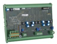
Addressable 4-analog-output module that delivers four analog 4-20mA signal outputs (detector output copy, min, max, average of a group of detectors) for connection to a datalogger, a PLC, a Building Management System (BMS), etc.
