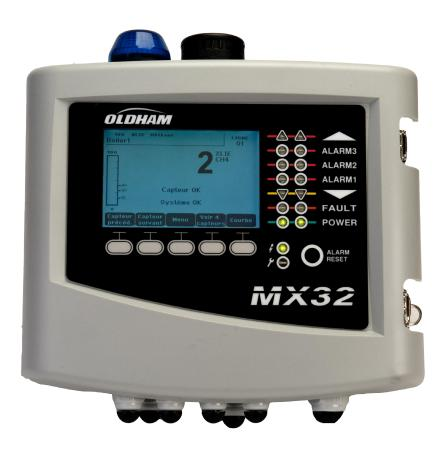
The MX 32 is a compact, low-profile controller that continuously monitors gas detection, including 4-20 mA, dry logic input, MODBUS RS485 signal from compatible detectors.
