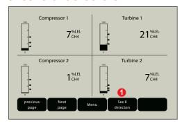
1Up to eight detectors displayed simultaneously
