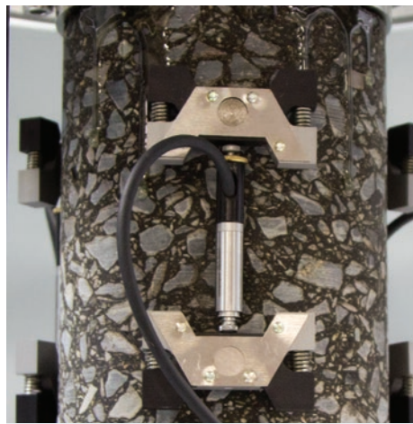
Uniaxial Fatigue – Unconfined
