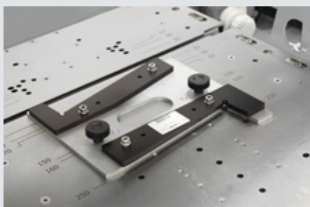
Trapezoidal specimen jig for two point bend
