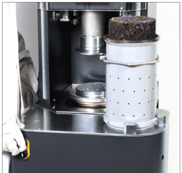
Integrated worktop with electromechanical extruder 78-PV2520/15
