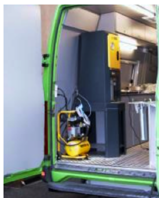
Gyrocomp installed inside a van as a road mobile laboratory
