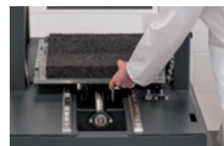
500 x 400 mm slab and lead rolled ball screw system
