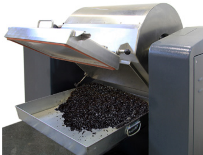
Detail of unloading: the mixing cylinder is rotated by a motorized tilting system for easy unloading. The tilting angle is adjustable to 130° to speed up the unloading operation.
