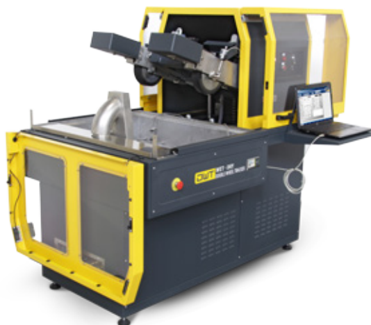
Detail of the sliding cover and motorized lifting system that rises the wheel assembly at the end of the test, making the use of the hoists obsolete
