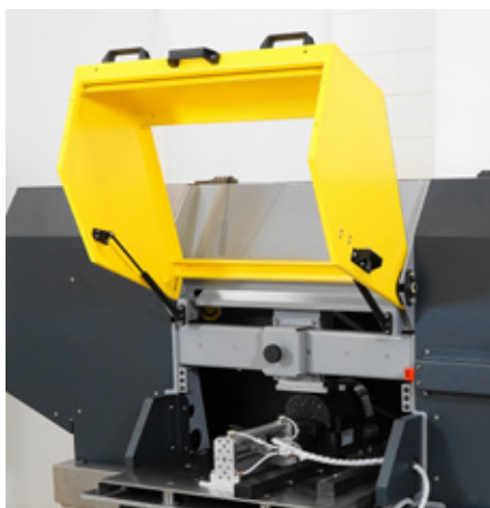
The protection cabinet ensures easy access for sample set-up, safe operation and protection from spray during cuts. Several automatic locking doors on the front, back and top prevent the operator from accessing the dangerous areas while the blade is running
