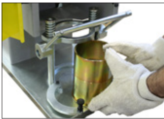
EN and ASTM compactors. Detail of clamping mechanism
