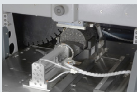
Automatic core docking jig for 100/150 mm diameter cores. For use with Autosaw II only
