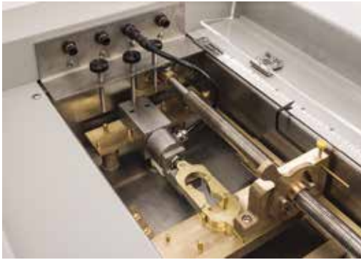
Interior of HA-1060 showing force determination transducer set up.
