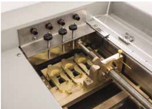
Interior of HA-1060 showing test molds, screw drive and disengage lever.
