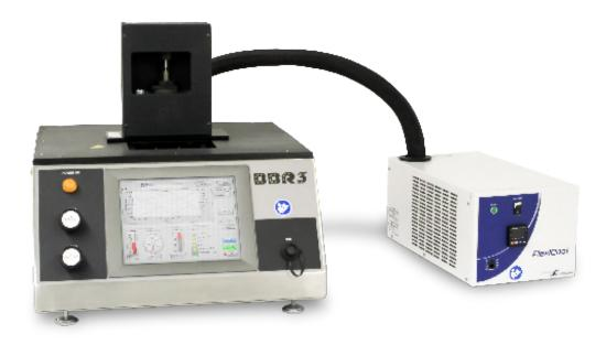
The ATS Bending Beam Rheometer 3 (BBR3) performs flexural tests on asphalt/bitumen binder and similar specimens per AASHTO T 313, AASHTO TP 87, ASTM D6648, and BS EN 14771 specifications as part of the PG grading system according to Superpave. An ATS original, the BBR3 is the first of its kind to offer a state of the art internal computer system, incorporating intuitive new software and touchscreen technology.
