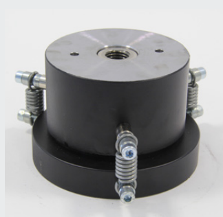
Detail of upper platen and spherical seat strictly conforming to ASTM C39 and AASHTO T22
