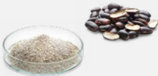
Homogeneous sample: Beans before and after grinding with the Variable Speed Rotor Mill PULVERISETTE 14
