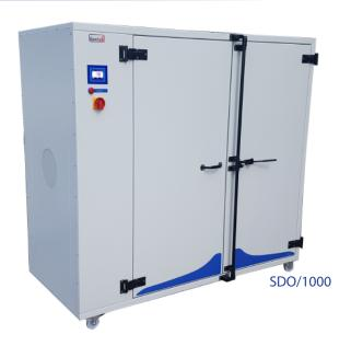
The Genlab range of Soil Drying Ovens offers a selection of highly efficient, reliable and cost effective units to suit most material testing requirements. These range of ovens are designed for drying large quantities of soils and aggregate samples and maintains temperature in accordance with BS EN and ASTM requirements. They feature our latest touch screen control system, which offers intuitive control and excellent accuracies designed for soil drying ovens.
