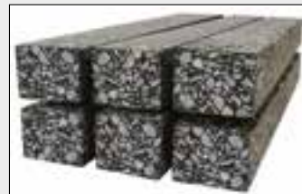
- Up to six 50mm wide prismatic specimens
