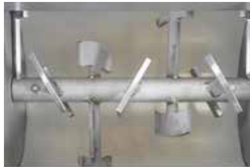
Detail of drum with helical mixing shaft
