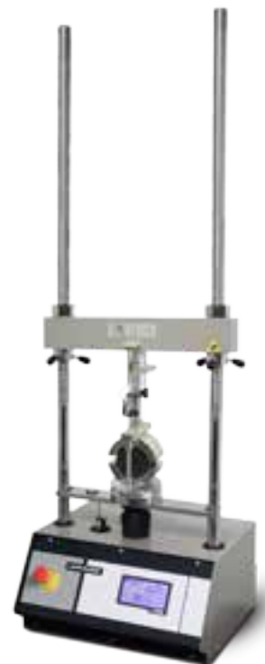
UNIFRAME 70-T1192, 100 kN cap. equipped with Marshall digital testing accessories
