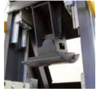
Detail of segment head incorporating vibration unit
