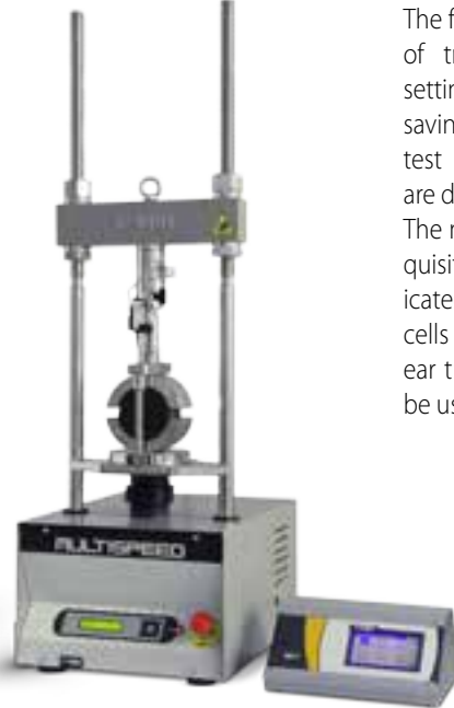
34-V1072 With Marshall test accessories (Digital mode)
