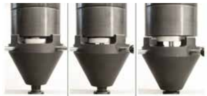
Detail of the weight positioning system showing, from left to right, no-load phase, pre-load phase (25 N) and load phase (525 N). The system allows transition from the no-load to the pre-load phase, then to load phase in a very fast, precise and
