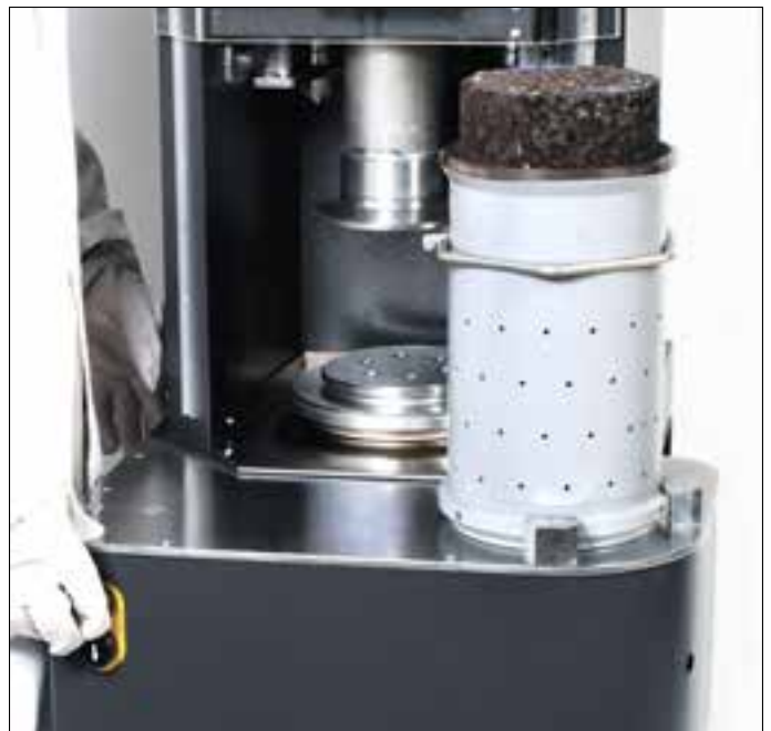
Integrated worktop with electromechanical extruder 78-PV2520/15
