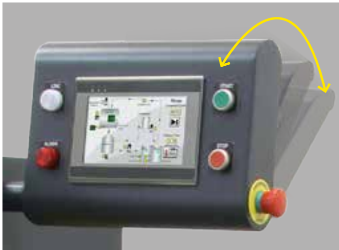
7" touchscreen swinging panel displays the operating stage and recorded data.
