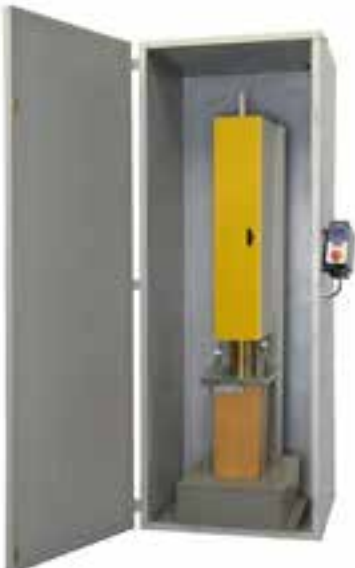
Noise reduction and security cabinet for automatic Marshall ASTM and EN compactors model 76-B4000/CB
