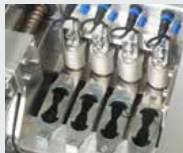
Detail of load cells and briquette moulds of High performance and Research ductimeters
