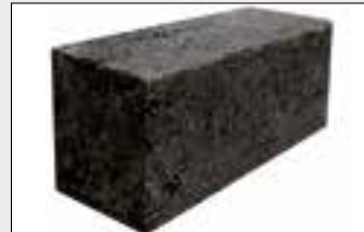
- Prismatic specimen produced by the PreSBOX
