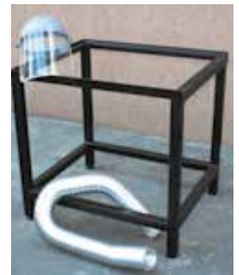
Exhaust pipe (supplied with the binder analyzer), metal stand and face shield (accessories)
