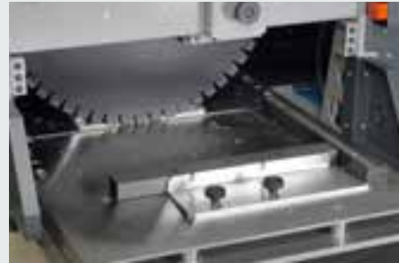
Jig for prisms and slabs
