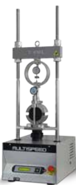
34-V1072 With Marshall test accessories (Analog mode)
