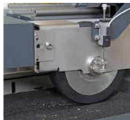
Detail of the testing wheels with rut depth measurement transducers axially mounted in alignment with the wheels centre
