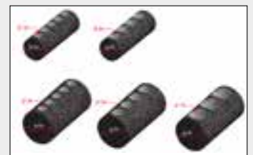
- Many cylinder samples can be cored from the cylindrical specimen using the Multi Core-Drill
