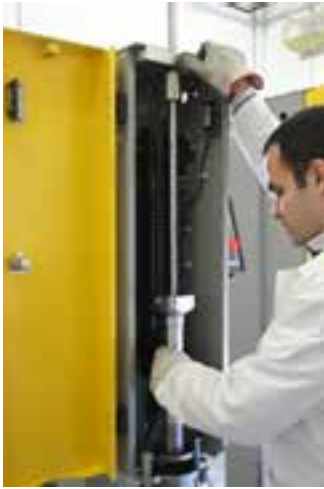
EN and ASTM compactors. Detail of lifting mechanism.
