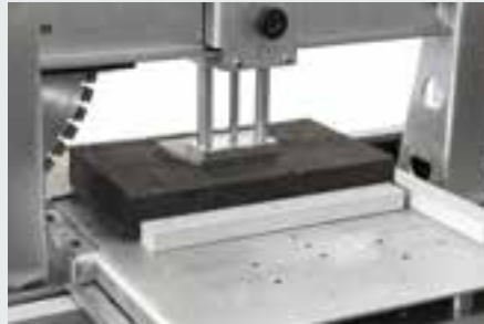
Clamping device for slabs included in Autosaw II and Multisaw
