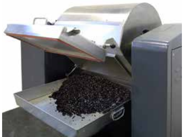
Detail of unloading: the mixing cylinder is rotated by a motorized tilting system for easy unloading. The tilting angle is adjustable to 130° to speed up the unloading operation.
