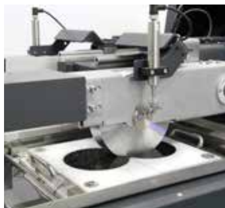
Detail of the testing wheels with rut depth measurement transducers axially mounted in alignment with the wheels centre
