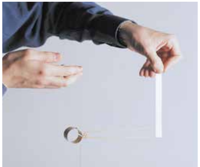
Use of the extensibility of mould apparatus 62-L0025/4, included with 62-L0025/B kit
