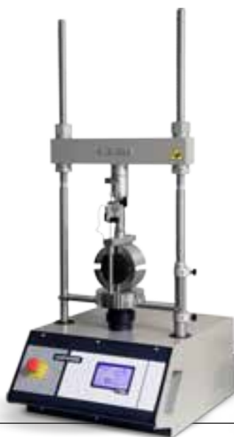
70-T1182 with accessories to perform the Marshall test
