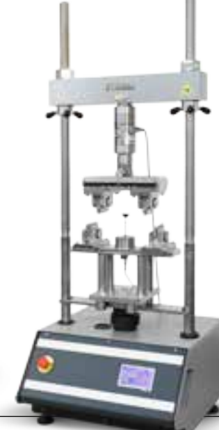
70-T1192 with accessories to perform flexure test on glass-fibre reinforced cement to EN 1170-5
