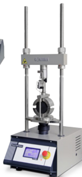
MULTISPEED 34-V1172 equipped with Marshall digital testing accessories
