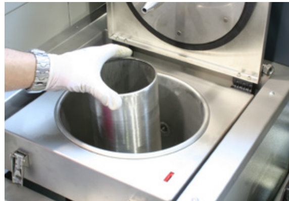
Placing the centrifuge cup into the centrifuge unit
