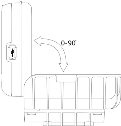
The display unit can be angularly adjusted from 0° to 90° for better viewing experience during measurement.
