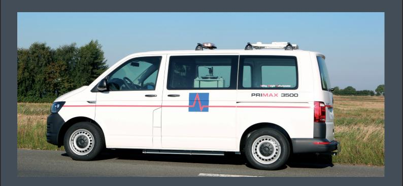
Sweco attaches great importance to supplying safe and stable equipment and the newest technology forms the basis of the FWD equipment. The PRIMAX software incorporates alarms that are displayed on the computer screen. If the operator ignores vital warnings, certain functions cannot be performed with the FWD e.g. in connection with pavement temperature measuring. The equipment cannot be driven to
